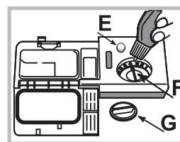
1. Open the dispenser by turning the cap "G" in an anticlockwise direction.
