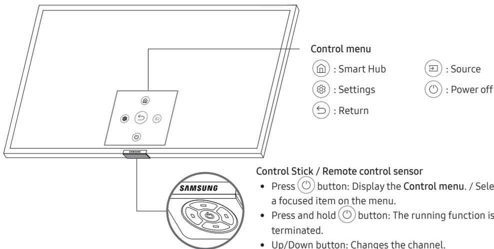
The Control Stick is located on the bottom of the TV.
